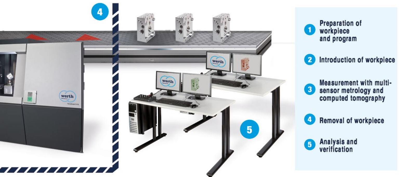
Network of Werth ScopeCheck® S and TomoScope® FQ for inline measurements with multisensor technology and computed tomography in 30-second cycles
