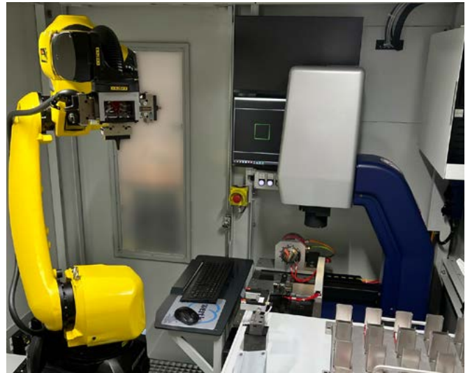
View of the measuring cell with ScopeCheck® S and robot
