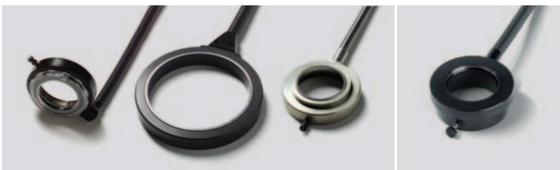
**Customised solutions** for lightguides in response to customer's special requirements, e.g. 66 mm continuous ringlight with 90° angled lightguide and focusing attachment or maxi-ringlight with 188 mm internal diameter. Continuous ringlights 66 mm are also available in **ESD versions** (without focusing attachment), i.e. any charge that may occur will be dissipated via/through the light source.
