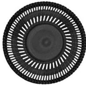
Cutting head of an electric razor with 48 Gvoxel – voxel size 1 µm
