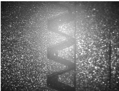
Interfering reflection when measured with brightfield incident light
