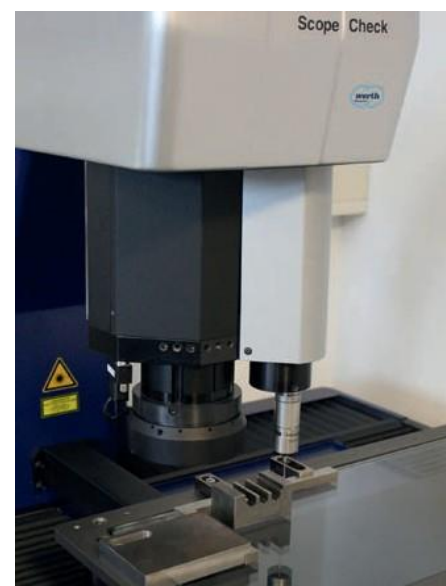
For tactile measurements, the components must be properly clamped to prevent them from moving. The fixtures are later used for process control in production as well.
