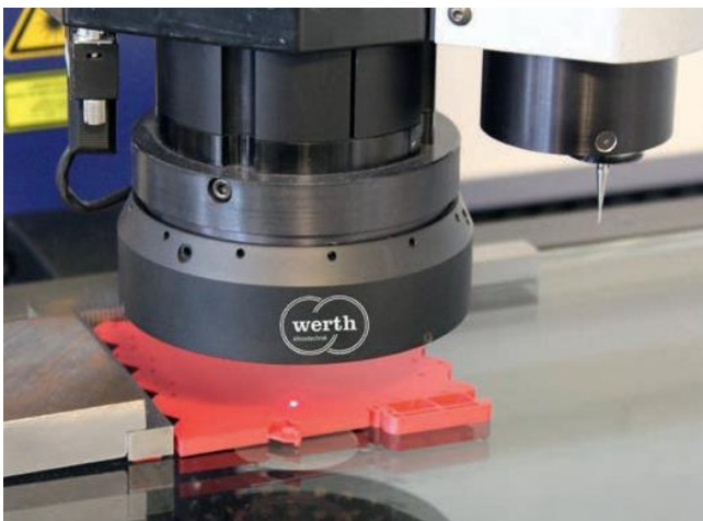
Measuring the flatness of plastic sheets. The laser on the 3D multisensor coordinate measuring machine reduces the inspection time by about two-thirds.
