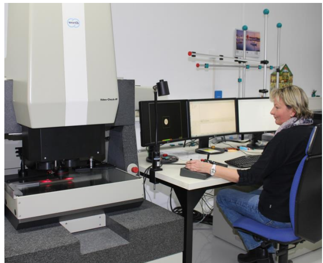
The fixed portal measuring machine is equipped with telecentric optics as well as a fiber probe and a conventional trigger probe.
