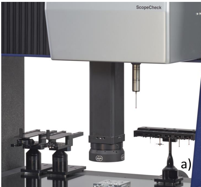
ScopeCheck® FB DZ with two independent sensor axes for collision-free measurement in the production environment: a) image processing sensor in use; b) scanning probe in use – the changing racks for the multisensor systems and the probe styli are in the background
