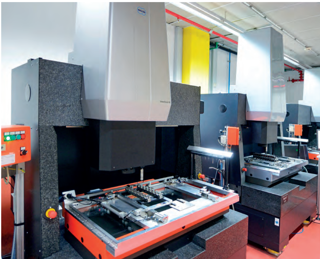
For high-precision measurement tasks: the highest-precision class of VideoCheck® machines can reach a maximum permissible error in the range of tenths of microns.
